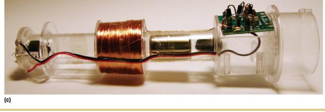
Figure 3. Commercial inertial-power scavengers. Two mechanisms for self-winding electric watches—(a) the ETA Autoquartz design and (b) the Seiko AGS (Automatic Generating System) generator for the Kinetic series—and (c) an inertial solenoid generator from a commercial shake-driven light-emitting-diode flashlight. (diagrams courtesy of the Swatch Group and Seiko Epson)
