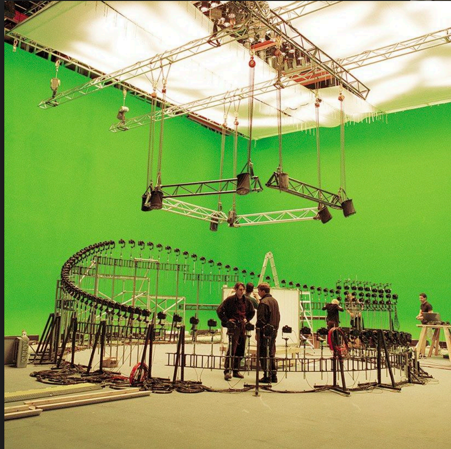
99 Camera "Bullet time" rig from The Matrix
