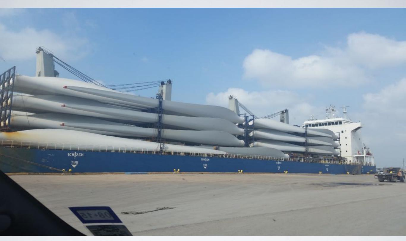
"Ninety individual blades, each of them 128 feet long and weighing 77,000 pounds, were offloaded from the Chinese freighter 'Gong Yin 1' at the port and are now being loaded onto railcars. The blades were manufactured by Vestas Wind Systems, a Danish company, and are bound for a terminal in Manly, lowa, that handles wind turbine components. The blades are composed of carbon and glass fiber."
