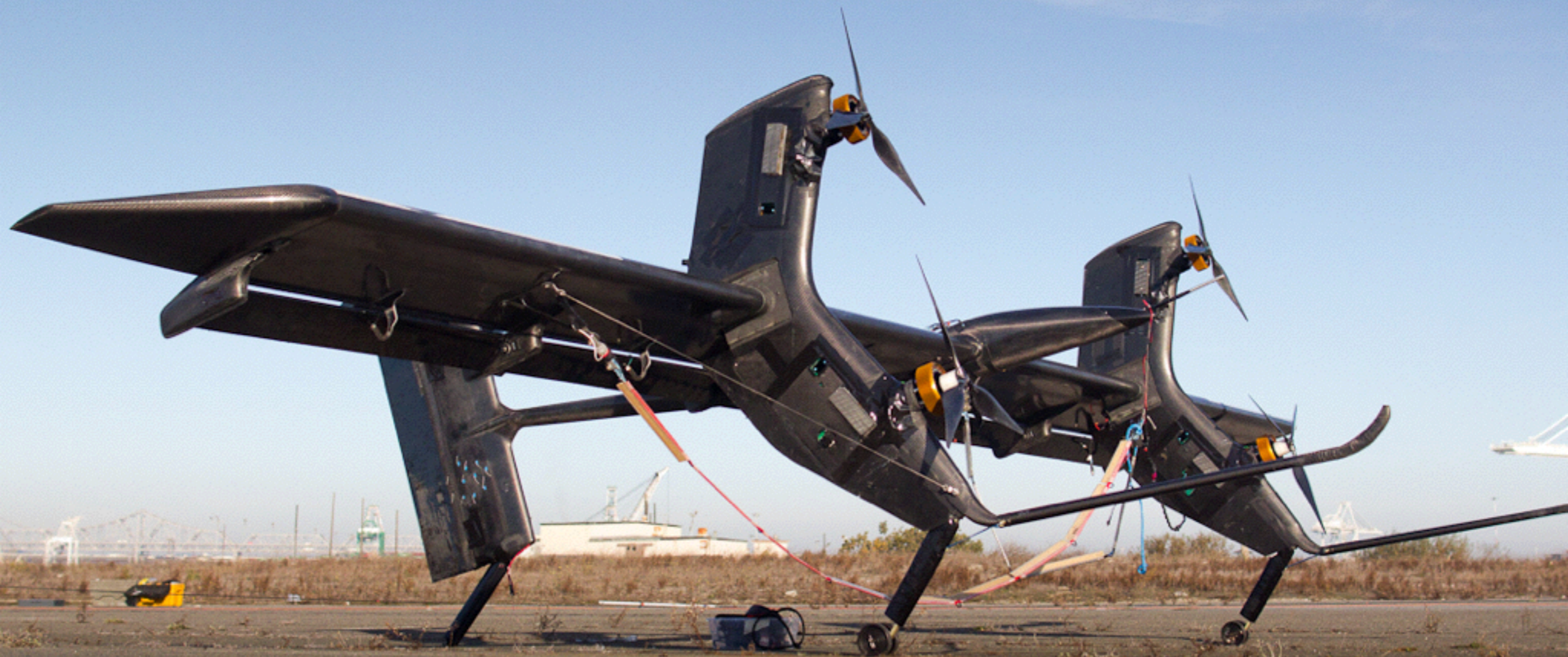
Makani M30 30kW prototype airborne turbine
