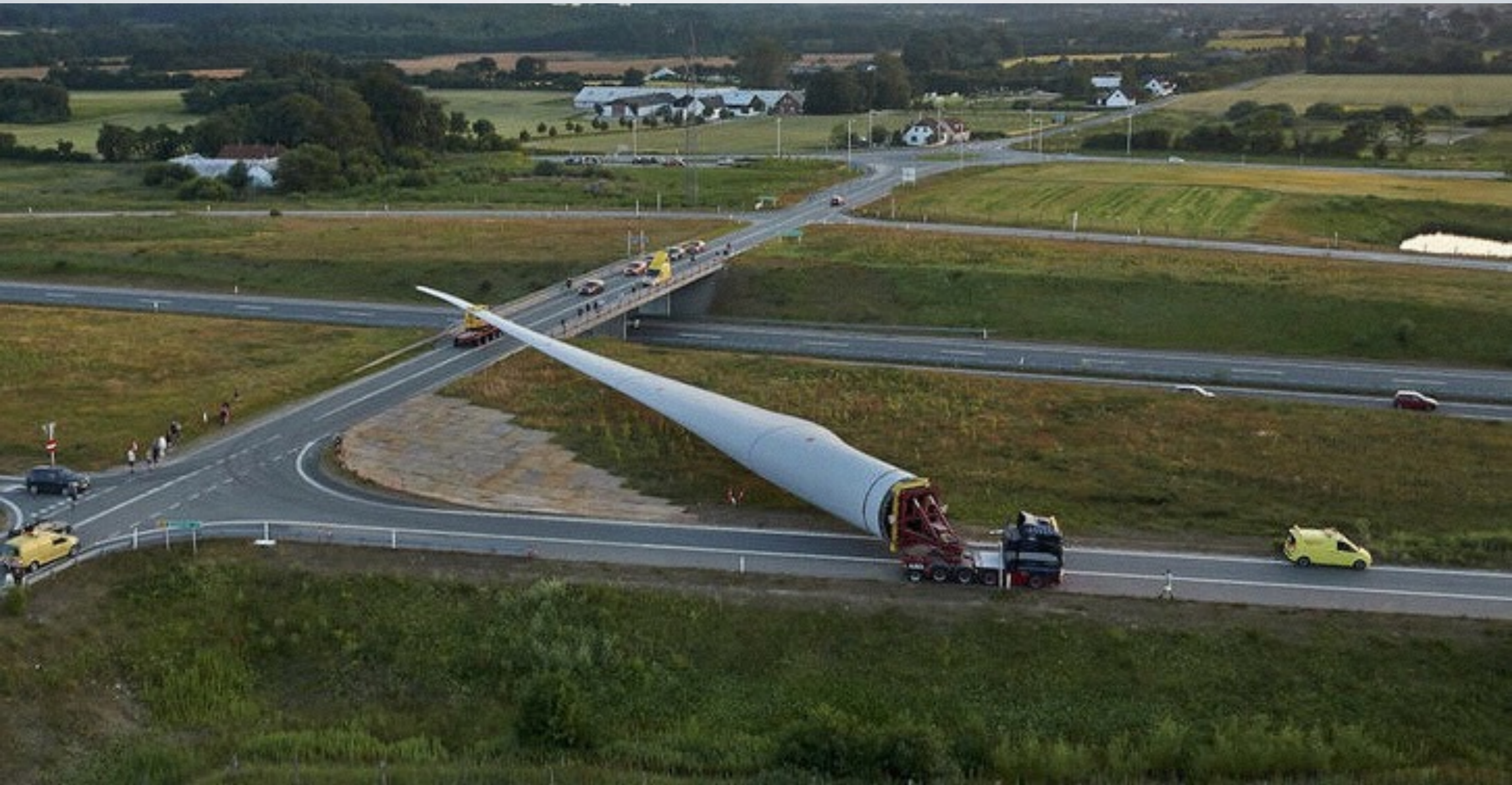
An 83.5-m-long blade made by Denmark's SSP Technology in transit to Scotland in 2013. It was called the longest blade in the world at the time.
