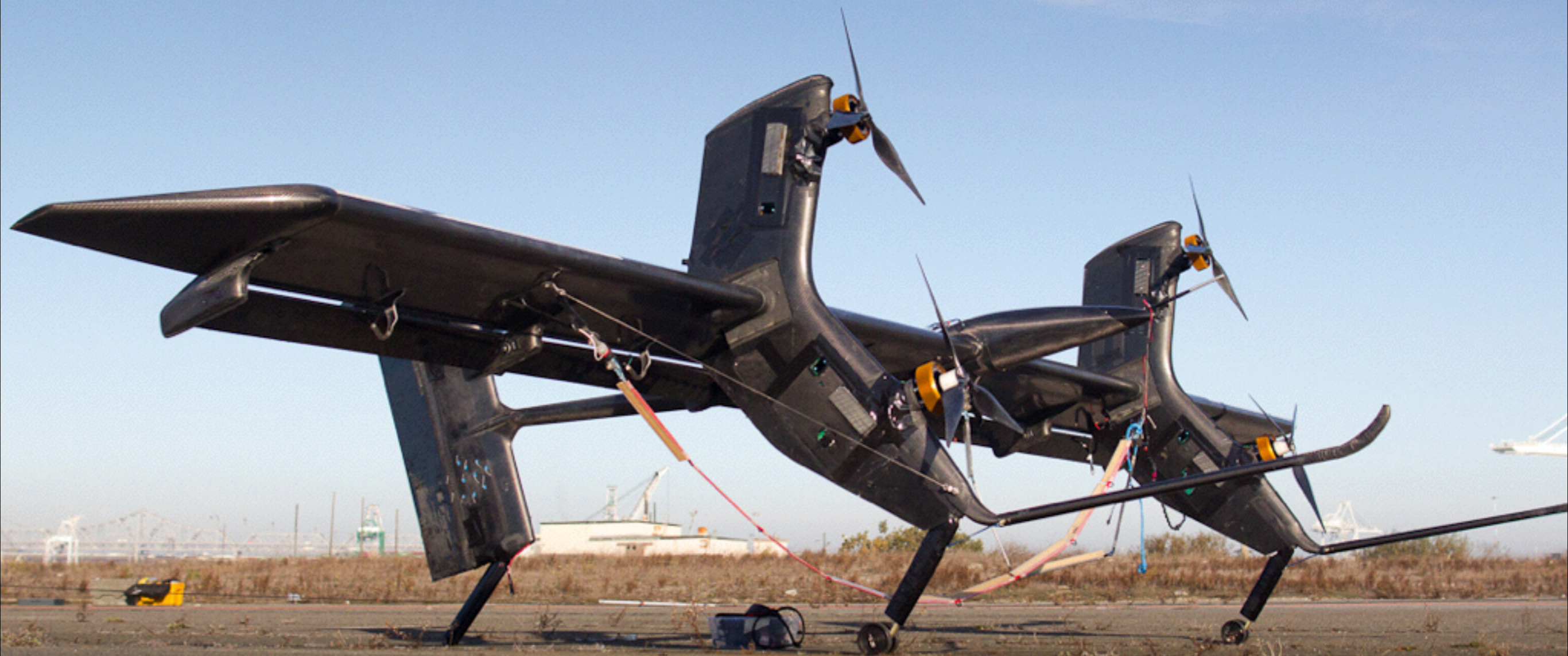
Makani M30 30kW prototype airborne turbine
