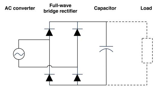
This is the basic circuit for converting an AC input to DC. The arrangement of four diodes is often depicted in a diamond shape; the circuit is the same. As each diode has a **forward voltage Vf** our DC output will be less than our AC input by at least *2Vf*. Schottky diodes have low forward voltages.
